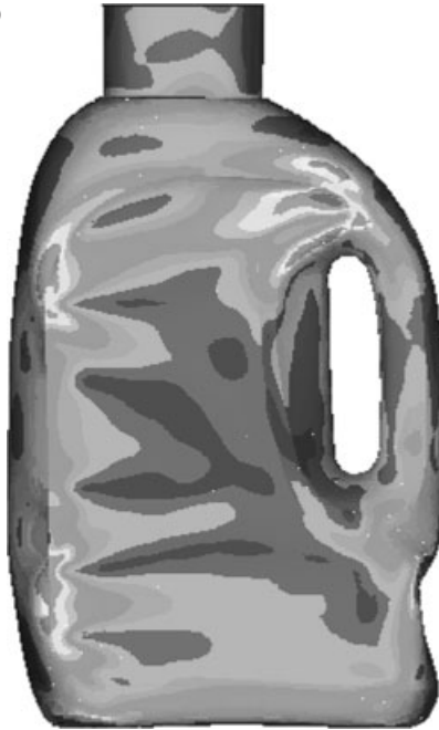
Figure 11.7. (a) Top load test and (b) analysis contour plot.
